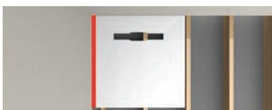
**Step 5.** Trim up to 50mm from any former edge to avoid joist/obstructions if necessary.
