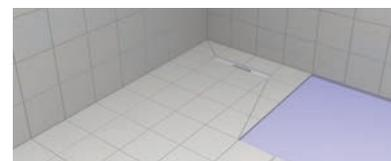
**Step 14.** Bed tiles on a suitable solid flexible tile adhesive – not notched - checking falls to channel. Use a flexible grout. Ensure channel top is 1 to 2mm below surrounding tiled surface.
