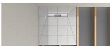
**Step 7.** Valley cut tiles to visible raised channel corners as required. See Figure A overleaf. Remove tiles for safe storage.
