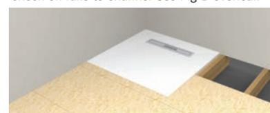
**Step 12.** Replace floor boards to former and secure. Lightly abrade former upper surface with 120 grit sand paper to aid tanking bonding.
