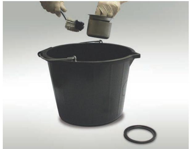
1. Remove crosshead screws from grating. Using appropriate gloves, grip the crossbar of the foul air trap and pull upwards making sure that the rubber sealing ring does not dislocate and fall into the drain. Remove sealing ring. Clean foul air trap thoroughly with soapy water.
