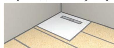
**Step 13.** Apply tanking tape, primer and liquid membrane to all joints and surfaces to manufacturers' instructions.
