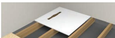
**Step 3.** Decide former orientation for optimum waste connection and falls. Any 90° rotation combination is possible.
